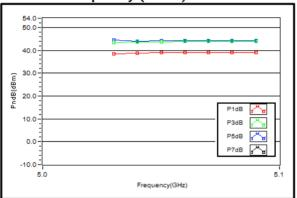
PSat vs. Frequency (Pulse)
